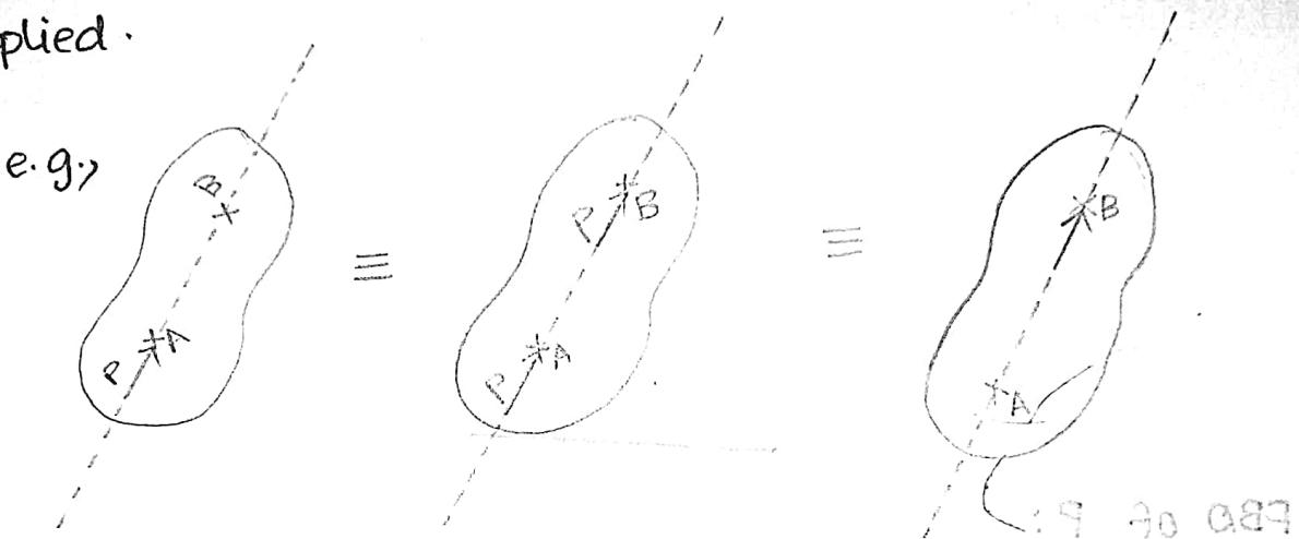
The force  $P$  acts on a rigid body at point A. According to the principle of transmissibility of forces, this force has the same effect on the body as a force  $P$  applied at point B along its line of action.
